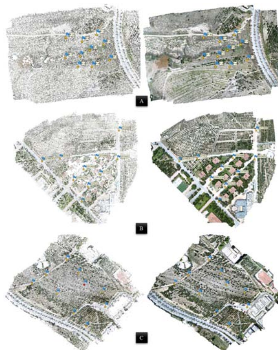
Figure 6. Sparse and dense point cloud (A: multi-sloping area, B: flat area, and C: sloping area, the left is the sparse point cloud, the right is the dense point cloud)
