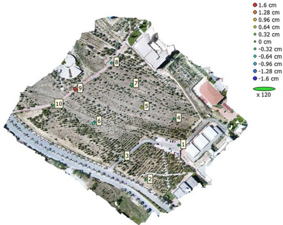
Figure 9. Point error distributions over a high-sloping area (1, 5, 6 and 9 Checkpoints)
