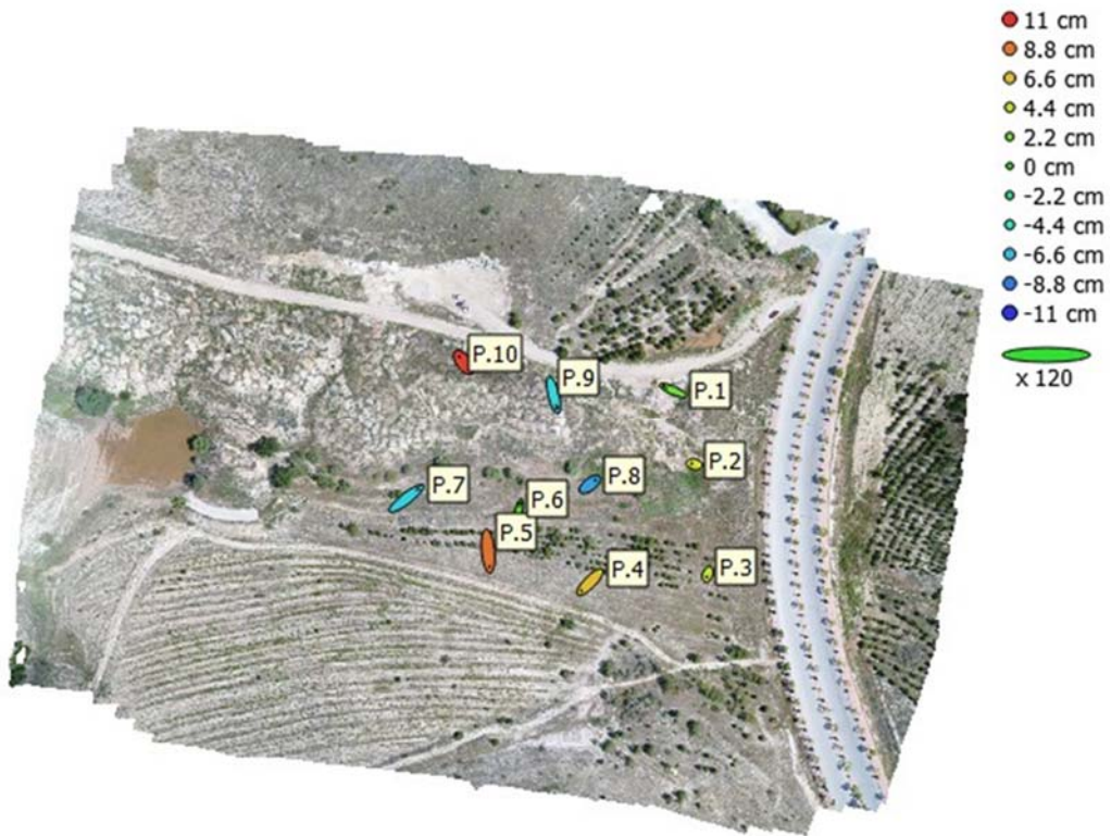
Figure 7. Point error distributions over a high-sloping area (P.1, P.6, P.7 and P.9 Checkpoints)
