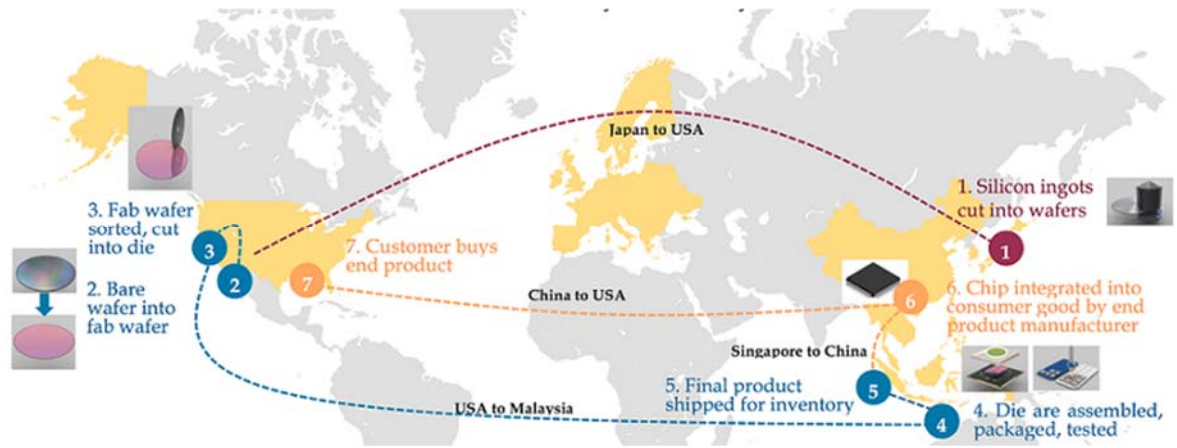
Figure 2. A typical IC production process example spans multiple countries [6]
